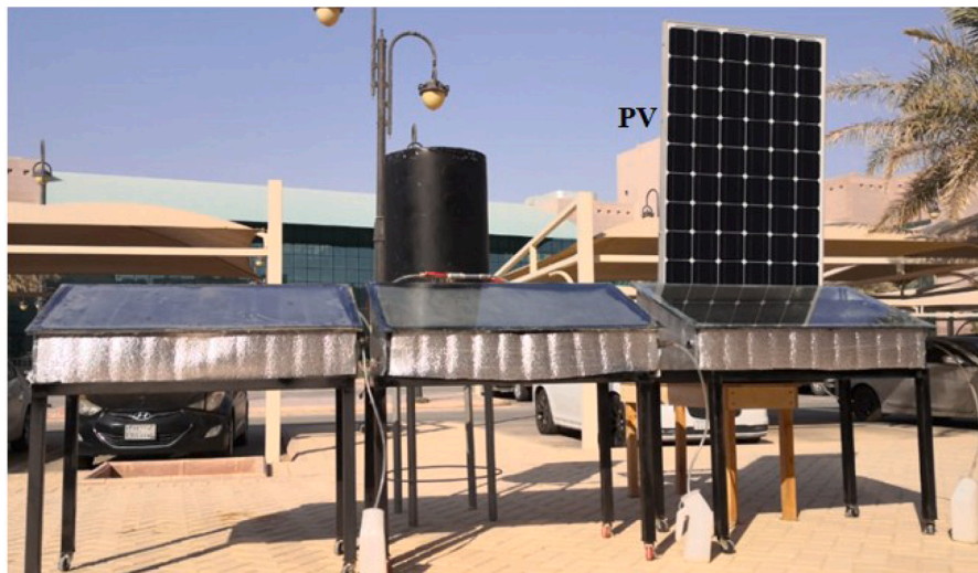
a. Conventional solar still b. Trays solar still c. Corrugated trays solar still
